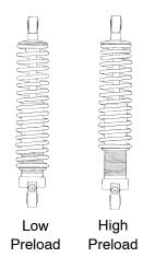
same. When decreasing preload, make sure at least two turns of preload are holding the spring between the retainer on top of the shock and the threaded spring preload adjuster nut on the shock body.
